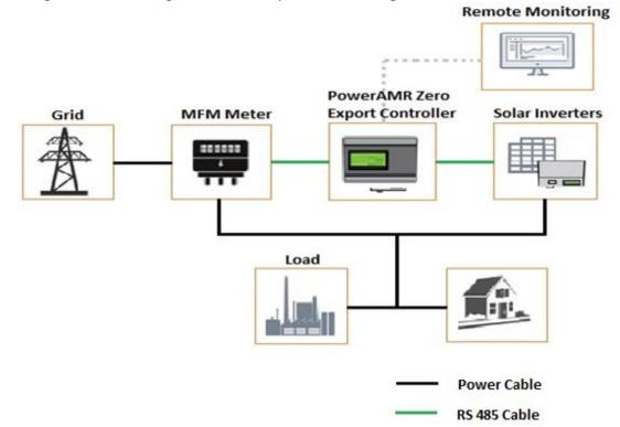
This solution is working when grid is available but there is no net metering at site. The zero export solution will help user to use solar as per demanded load. This solution will throttle the power of solar inverters as per building load and there will be No Export to grid.
